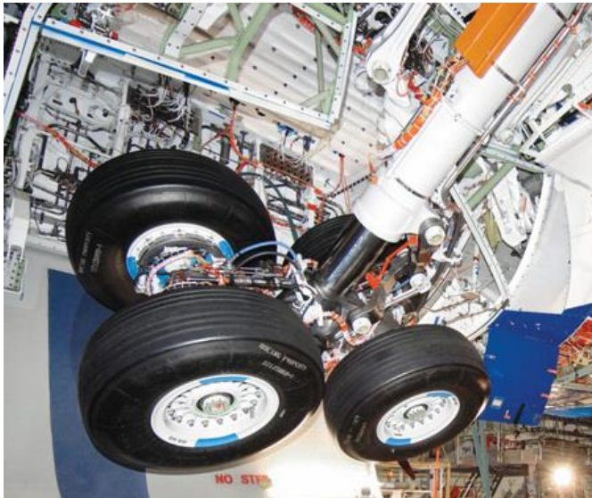
Landing gear testing (A380 @12 mio. cycles)
