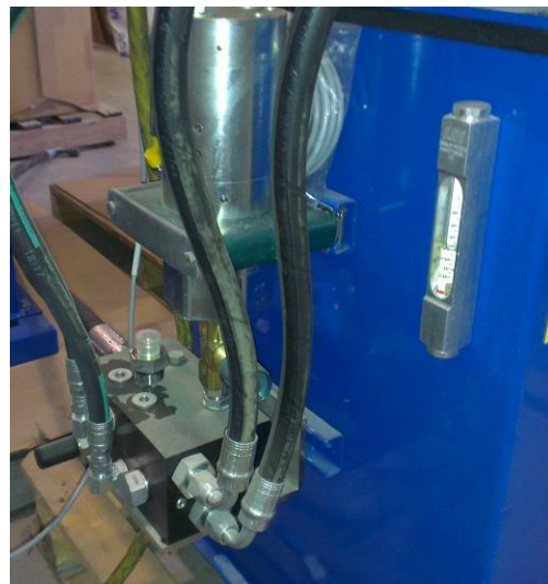
Bypass circuit for high flow applications:
